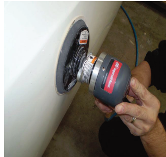
Dry sanding a vehicle can generate particulate matter
